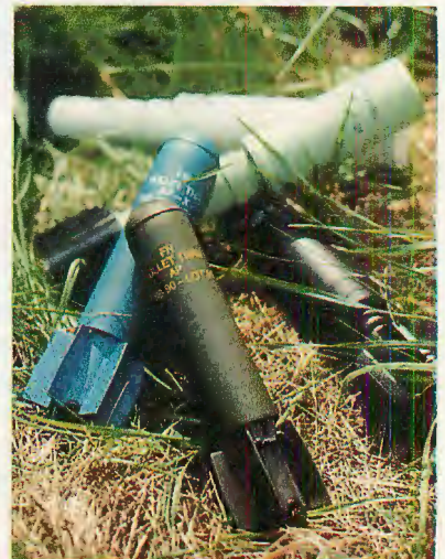
Munition types include an anti-personnel (AP) fragmentation round, an inert training (AP-X) round that is easily reusable, a non-telescopic white smoke (SMK) signal round and illuminating (ILL) parachute flares.
